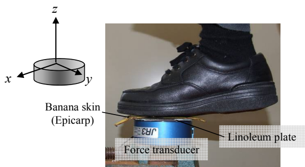
Fig. 2 Experimental set up with the coordinate of the detected forces
